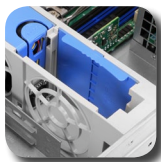
Air baffle to prevent air circulation
