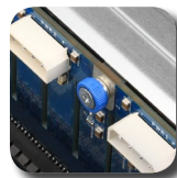
Tool-less backplane installation
