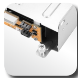
Tool-less ODD drive cage
